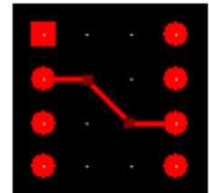
Corners can be dragged, inserted or deleted to change the trace's path. To insert a corner,
