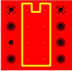
To look at the actual inner layer planes, select *View Power layer* or *View Ground layer* in the *Options* dialog box. This example shows pins 1, 3, and 8 connected to the Power plane. The other pads are isolated. You will notice that pins 1 and 8 are connected with *Thermal* pads, while pin 3 is connected with a *Solid* pad. Typically *Thermals* are used with pads connecting to a plane because they improve the solderability of the pad, reducing the chance of a "cold solder joint".
