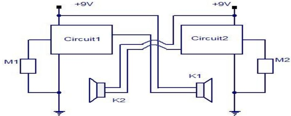
Transistor intercom connection diagram
