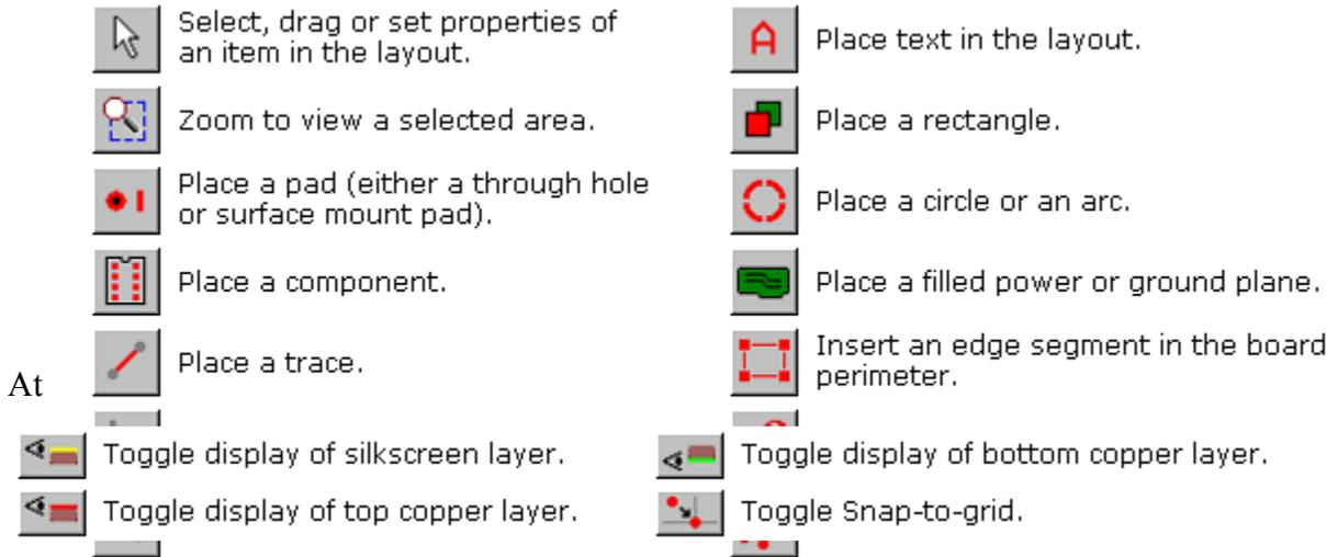
the bottom of the side toolbar are 4 additional buttons that toggle on and off features of the display:
